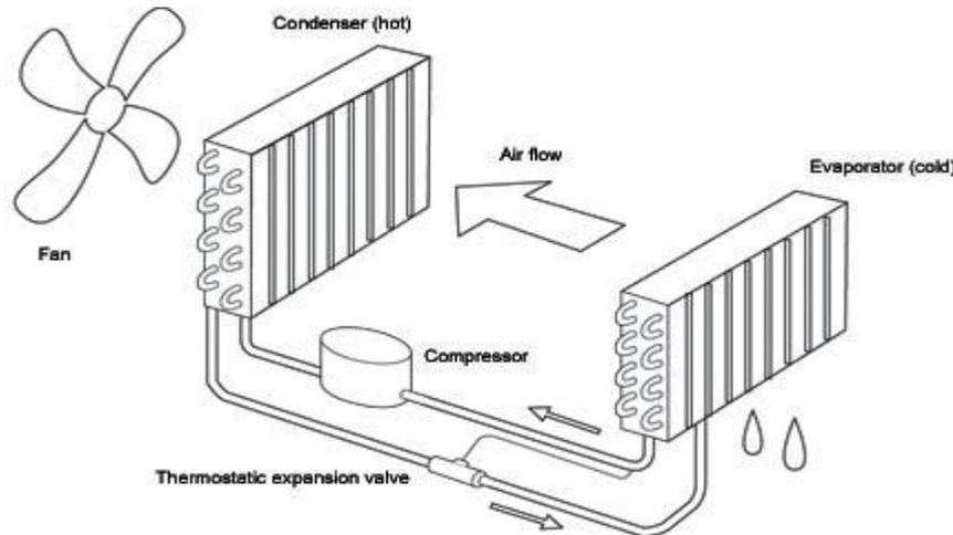
Figure-2. Dehumidifier thermodynamic cycle <https://physics.stackexchange.com/2019> (n.d).
