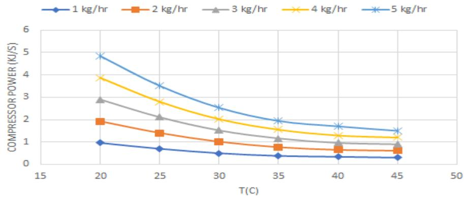
Figure-11. Compressor Power at different ambient temperatures.
