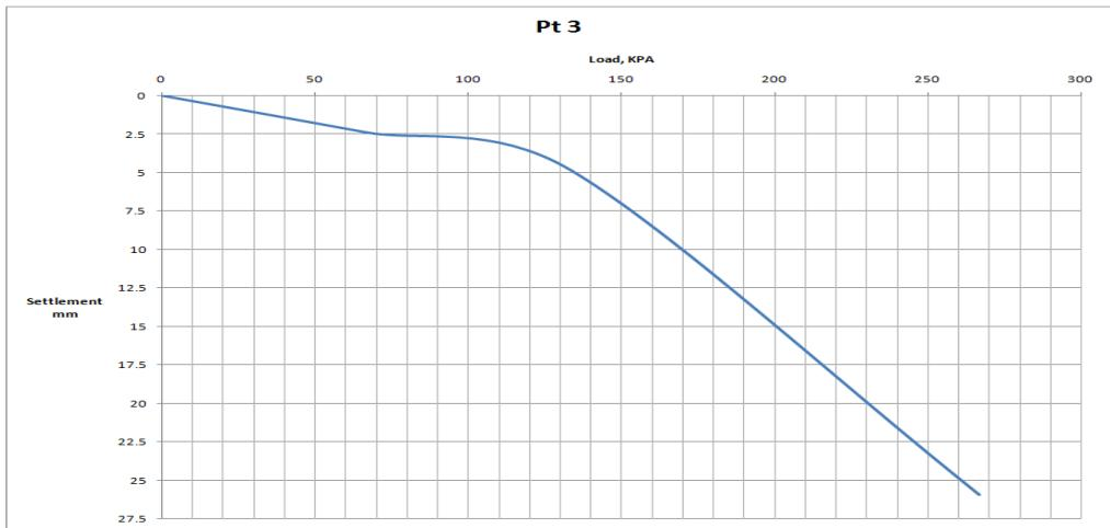
Fig-9. Loading settlement plot for point 3
