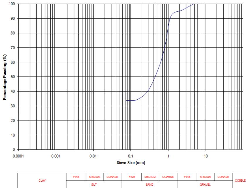
Fig-3. Particle size distribution curve in the area
