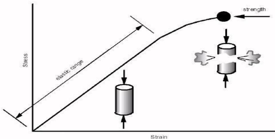
Fig-2. Stress-Strain Plot Showing the Elastic Range
