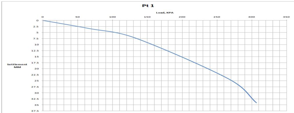
Fig-7. Loading settlement plot for point 1
