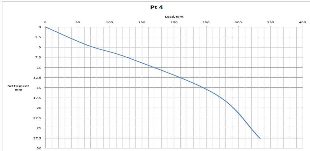
Fig-10. Loading settlement plot for point 4
