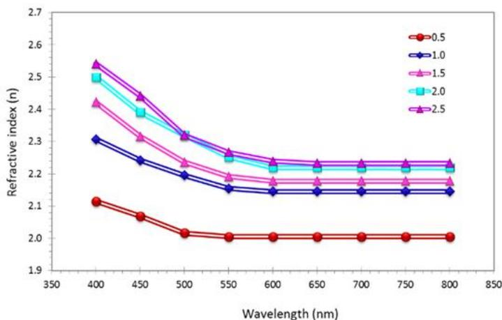
Fig-3. Refractive index of the ZrTiO<sub>4</sub> thin films
