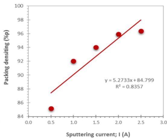
Fig-4. Packing density of ZrTiO<sub>4</sub> thin films
