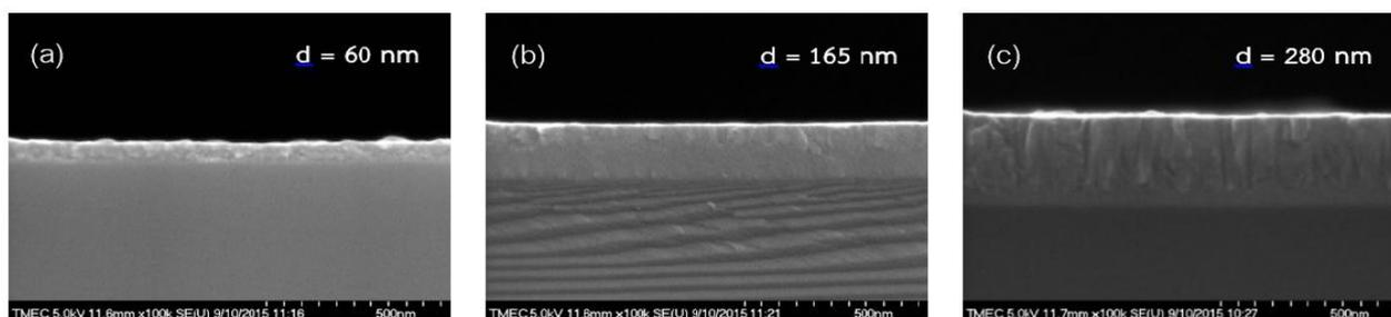
Fig-2. Cross-sectional FE-SEM morphology of the ZrTiO<sub>4</sub> thin films (a) 0.5 A, (b) 1.5 A, and (c) 2.5 A.
