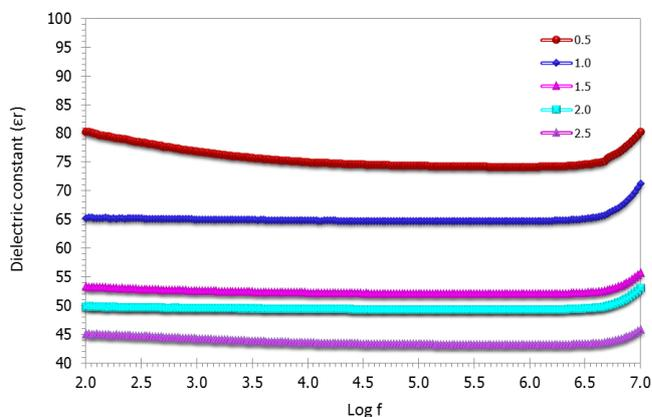
Fig-5. Dielectric constant of the ZrTiO<sub>4</sub> thin films
