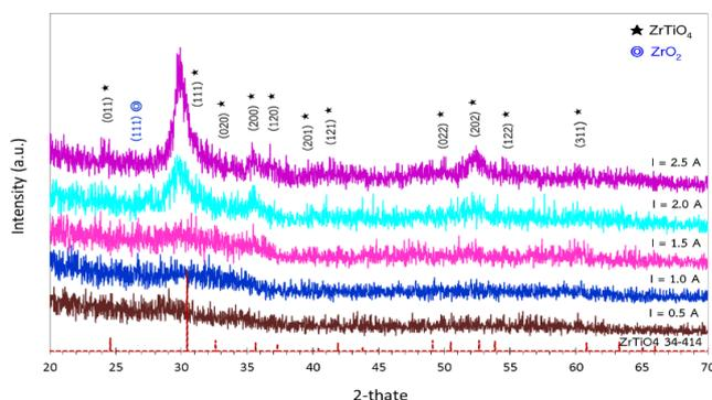
Fig-1. XRD patterns of the ZrTiO<sub>4</sub> thin films
