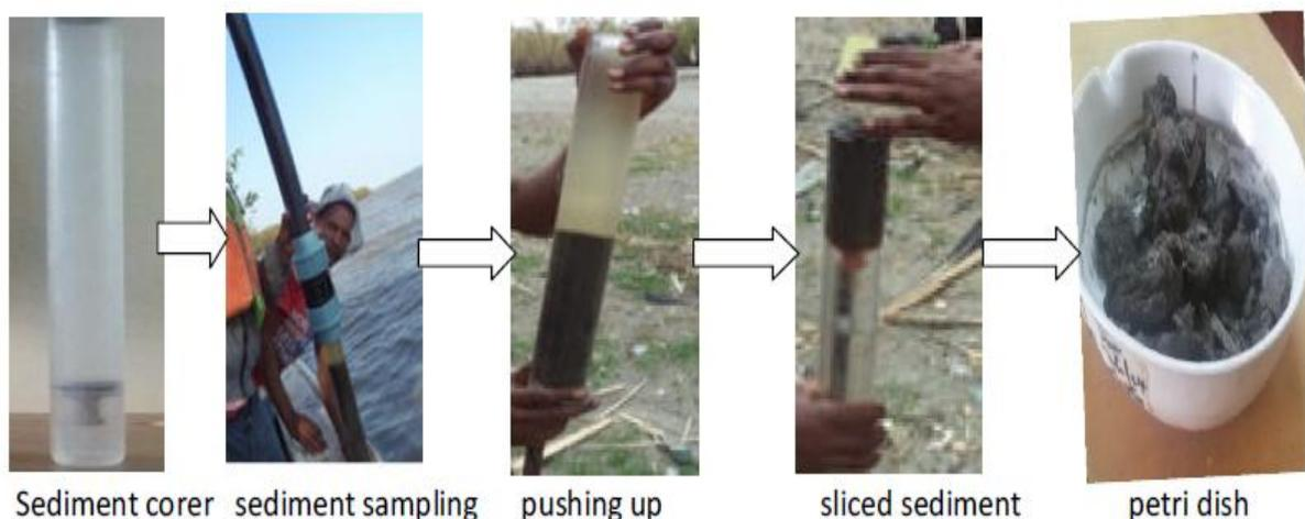
Figure-2. Sediment sampling producers using modified sediment corer.
