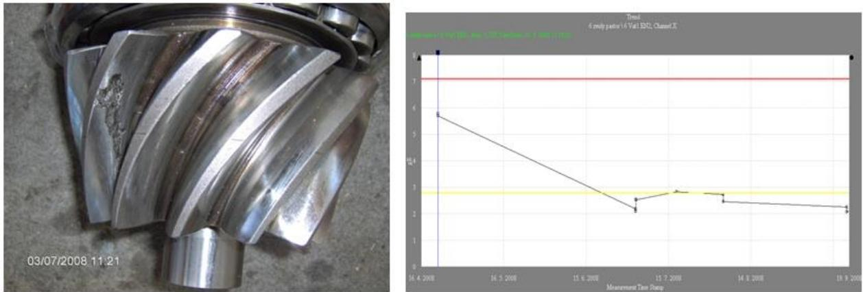
Fig-9. Damaged teeth of bevel gear and trend graph
