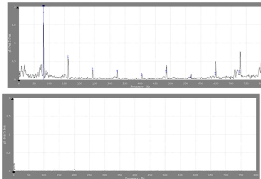
Fig-8. FFT spectrum before repair (EnvAcc=6.2gE), left, and after repair (EnvAcc=0.5gE)
