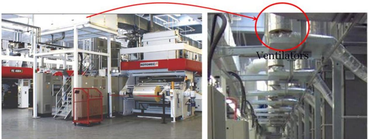
Fig-4. Flexoprinting machine and ventilators of drying section (right)
