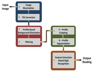
Fig-4. Steps Involved in the Proposed Algorithm for the Recognition of Seven Segment Numbers on Display Source: Kulkarni and Kute [12]
