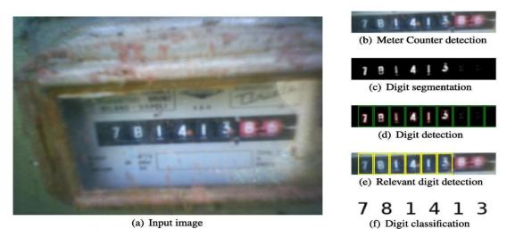
**Fig-3.** Results of the novel approach for automatic gas meter reading from the real world image **Source:** Vanetti, et al. [11]
