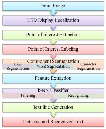
Fig-5. LED Text Detection and Recognition Process
