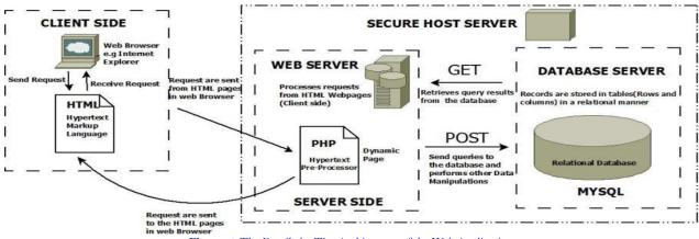
Figure-5. The Detailed 3 Tier Architecture of the Web Application
