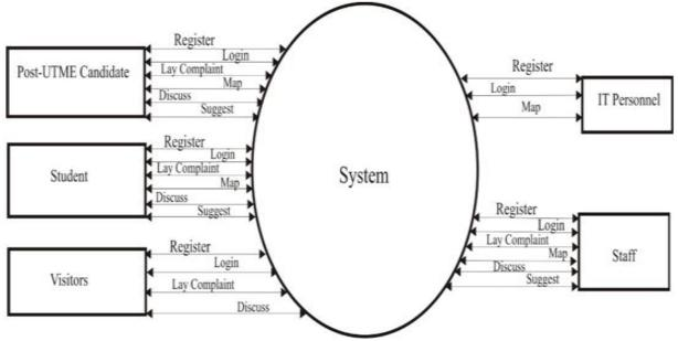
Figure-4. The System Context Diagram for the System
