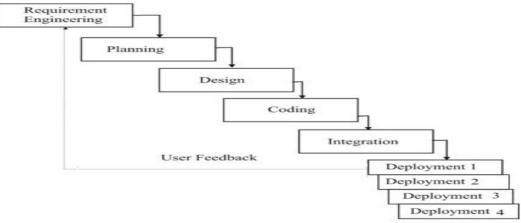
Figure-1. The Evolutionary Software Development Model (ESDM)
