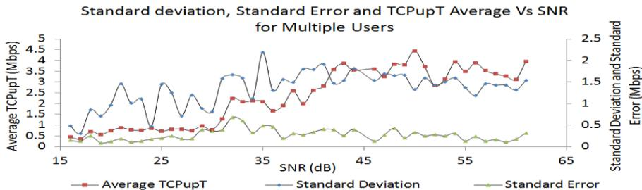
Fig-1. Standard deviation, Standard error and Average TCP<sub>up</sub>T values Vs. SNR for Multiple users
