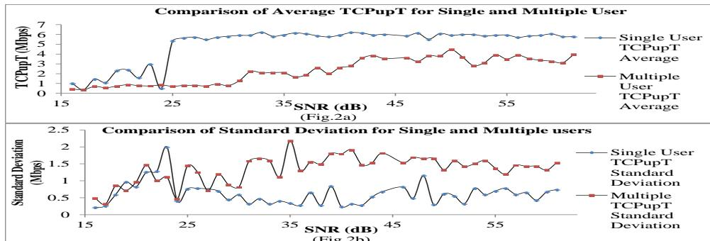
Fig-2. Comparison of TCP<sub>up</sub>T Graphs for Single and Multiple users on the network
