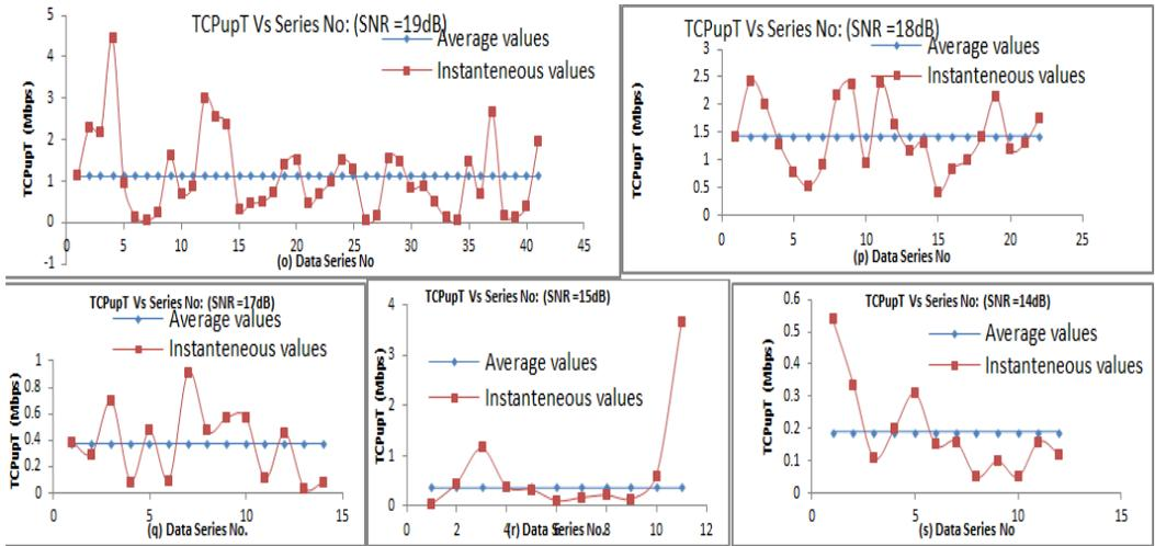
Fig-5. TCP<sub>up</sub>T variation about the mean for different SNR observed for single user scenario.
