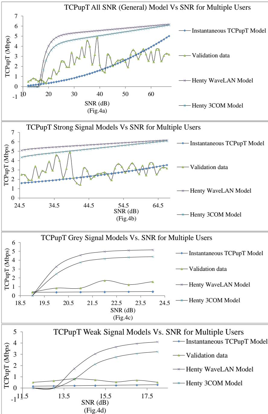
Fig-4. TCP<sub>up</sub>T Models compared with Validation data for different ranges of signals for multiple user scenario
