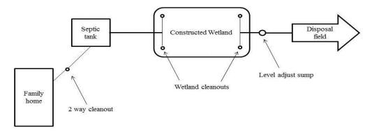
Fig-4. Schematic diagram of a wetland system
