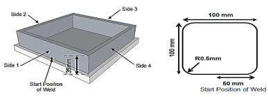
Figure-1. The Nominal WAAM CAD model and centreline tool path for the square sample
