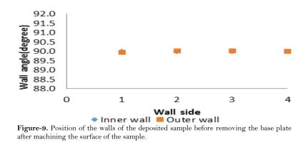
It can be seen from the graph that the walls of the deposited samples were straight due to the machining of both the inner and the outer surfaces. The base plate of this sample has, however, not been removed.
