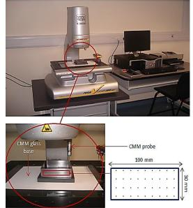
Figure-1. CMM machine setup for distortion experiment
