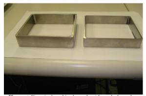
Figure-5. Deposited machined sample without the base plate
