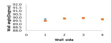
Figure-11. Position of the walls of the deposited sample after removing the base plate after machining the surface of the sample.
