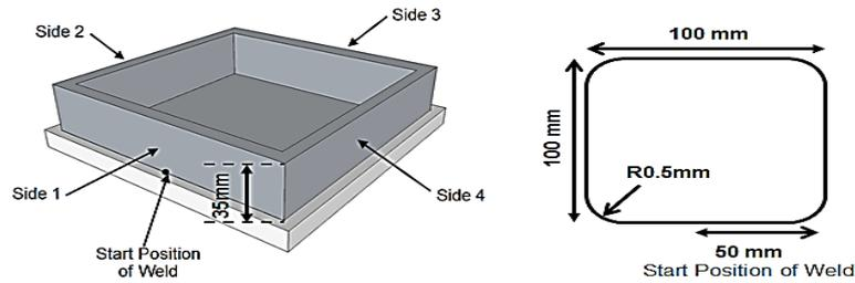
Figure-1. The Nominal WAAM CAD model and centreline tool path for the square sample
