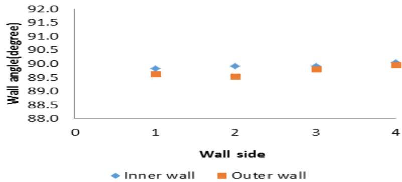
Figure-8. Position of the walls of the deposited sample after removing the base plate and left for 10 days (without machining the surface of the sample).
