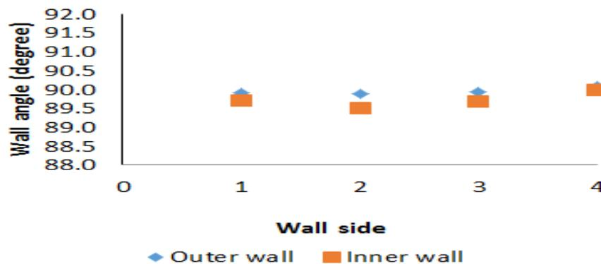
Figure-7. Position of the walls of the deposited sample after removing the base plate (without machining the surface of the sample)
