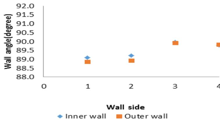
Figure-6. Position of the walls of the deposited sample with the base plate (without machining the surface of the sample).
