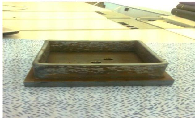
Figure-3. Deposited sample with the base plate without machining
