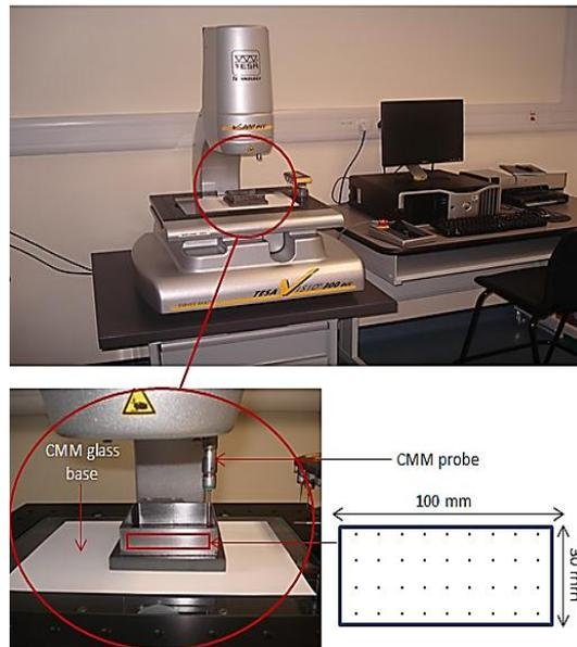
Figure-1. CMM machine setup for distortion experiment
