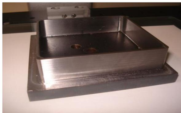
Figure-4. Deposited sample with the base plate after machining
