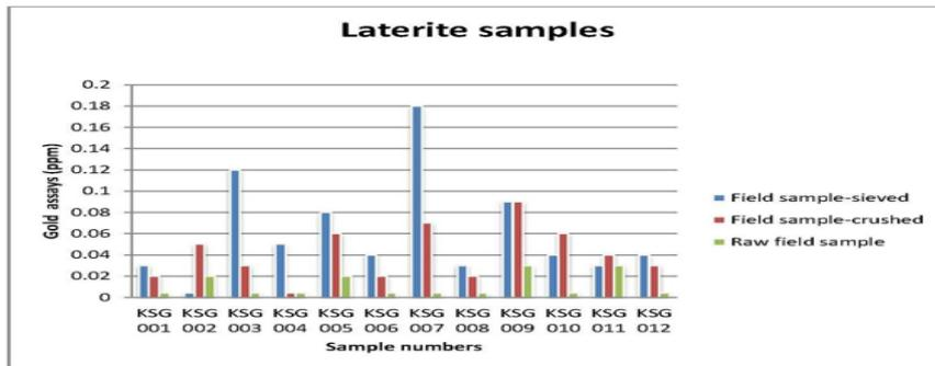
Fig-5. Comparison of Au assays in laterite samples prepared differently and analysed by FA-AAS to assess best sample preparation protocol for regional Au exploration
