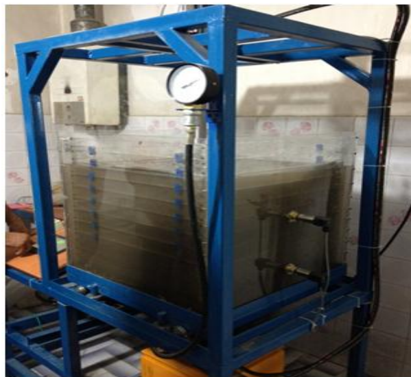
Figure-15. Physical modeling of cycle behavior for Anzali sand
