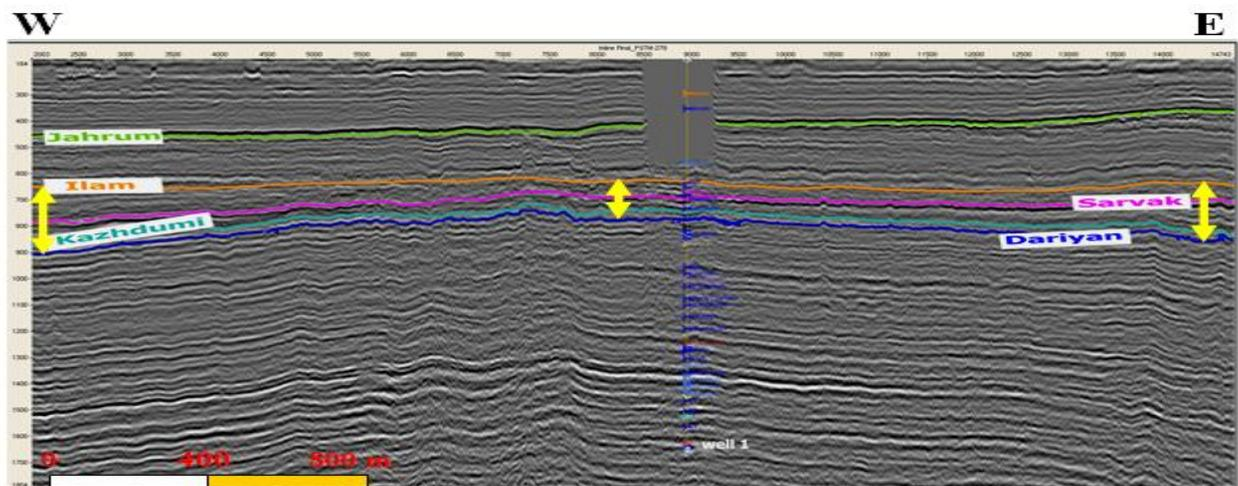
Fig-5. Seismic interpretation of Well 1 together with the information of studied headformations, (NIOC Company)
