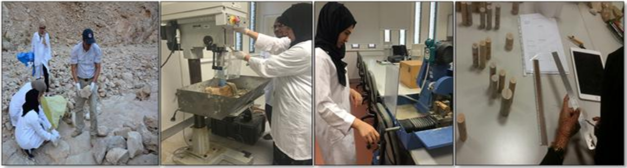
Fig-3. Sample collection and preparation (drilling, trimming and measurement).
