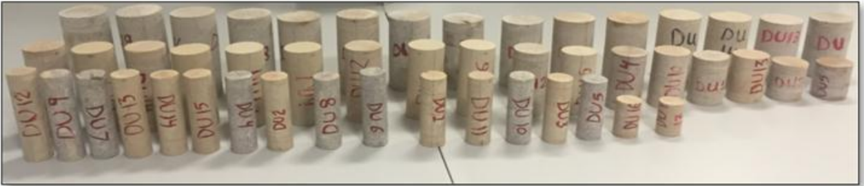
Fig-4. Core samples prepared and used in SV tests.
