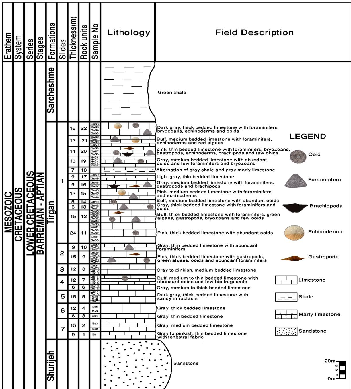
Fig-3. Stratigraphy of the Tirgan Formation in south flank of Ghorogh Syncline
