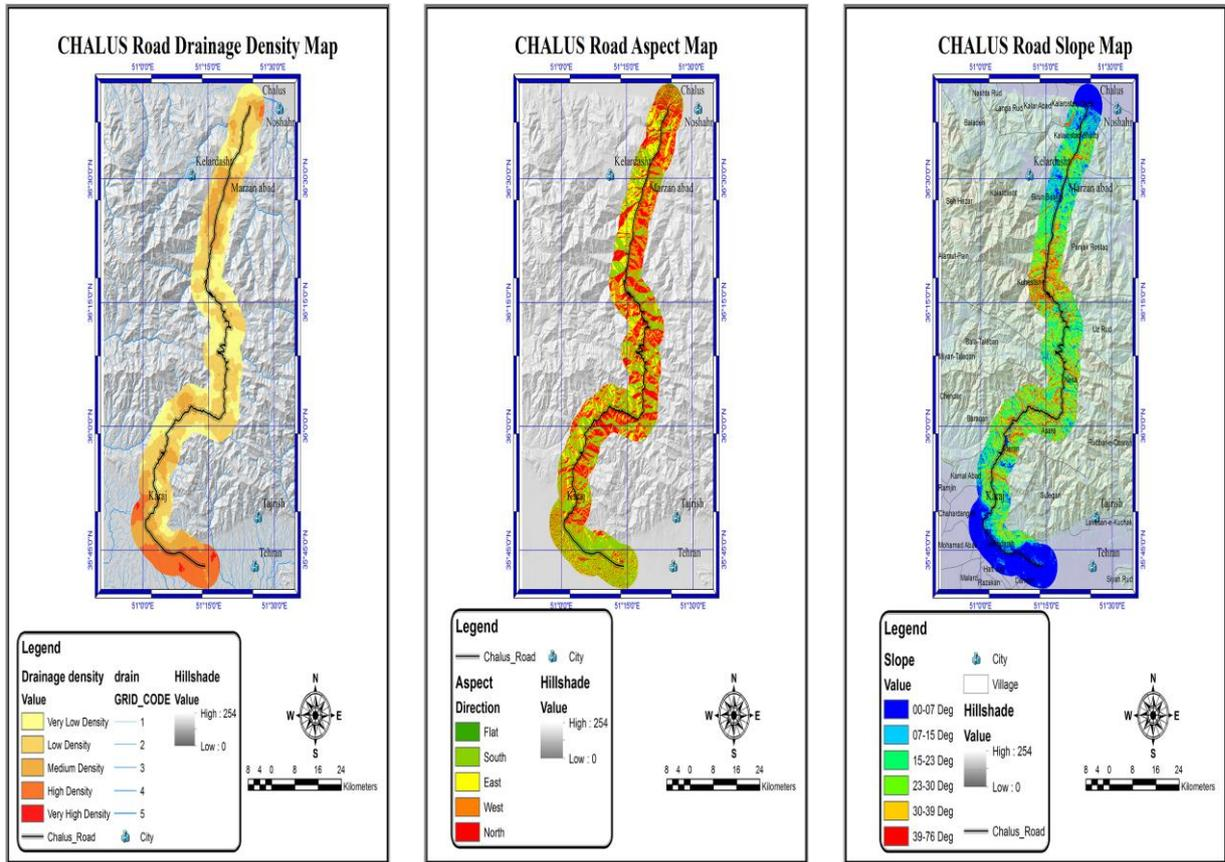
Fig-5. Drainage density, Aspect and Slope maps of Chalus road (Obtained from DEM and processed with GIS)
