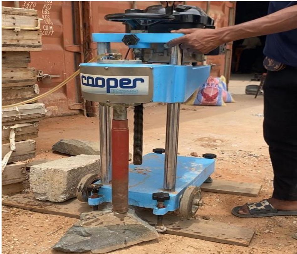
Figure 4. Image of coring machine showing a sampled rock being cored.
