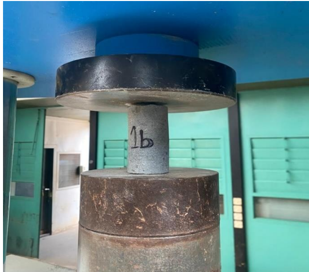
Figure 6. Image of rock core under uniaxial compressive test.
