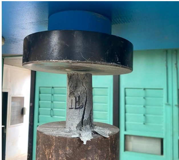
Figure 7. Image of failed core under uniaxial compressive test.
