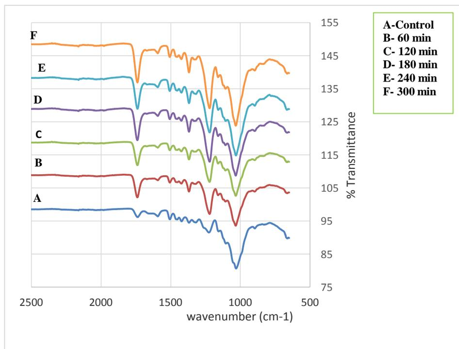
Figure-1. FT-IR (ATR) spectra of acetylated and untreated *Triplochiton scleroxylon* wood.
