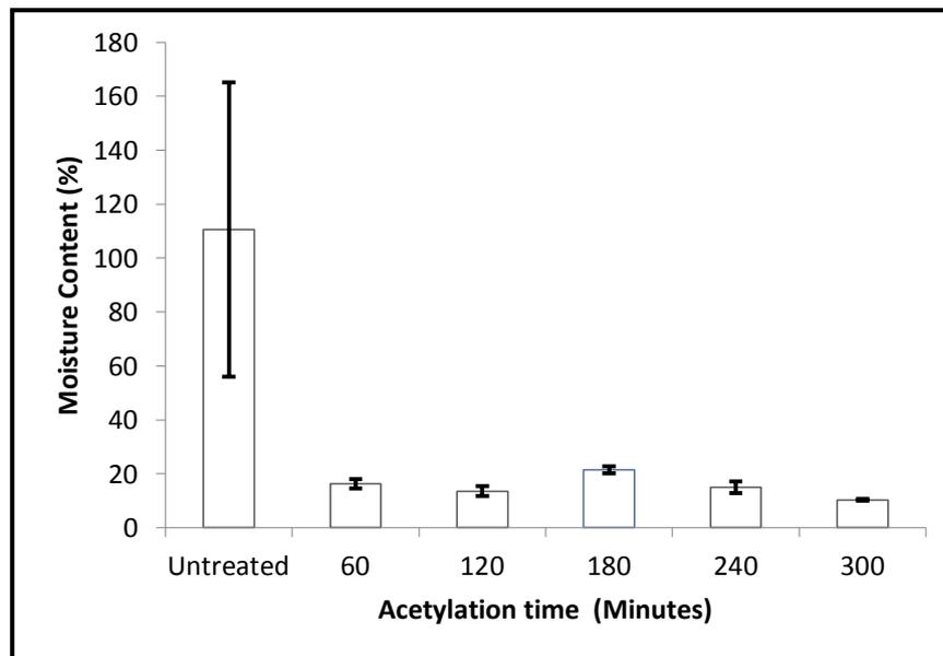
Figure-2. Moisture content of acetylated and unmodified *Triplochiton scleroxylon*
