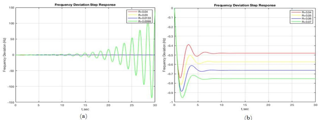
**Figure-1.** Frequency deviation step response for (a) different values of governor speed regulation (b) LFC under positively biased attack condition.
