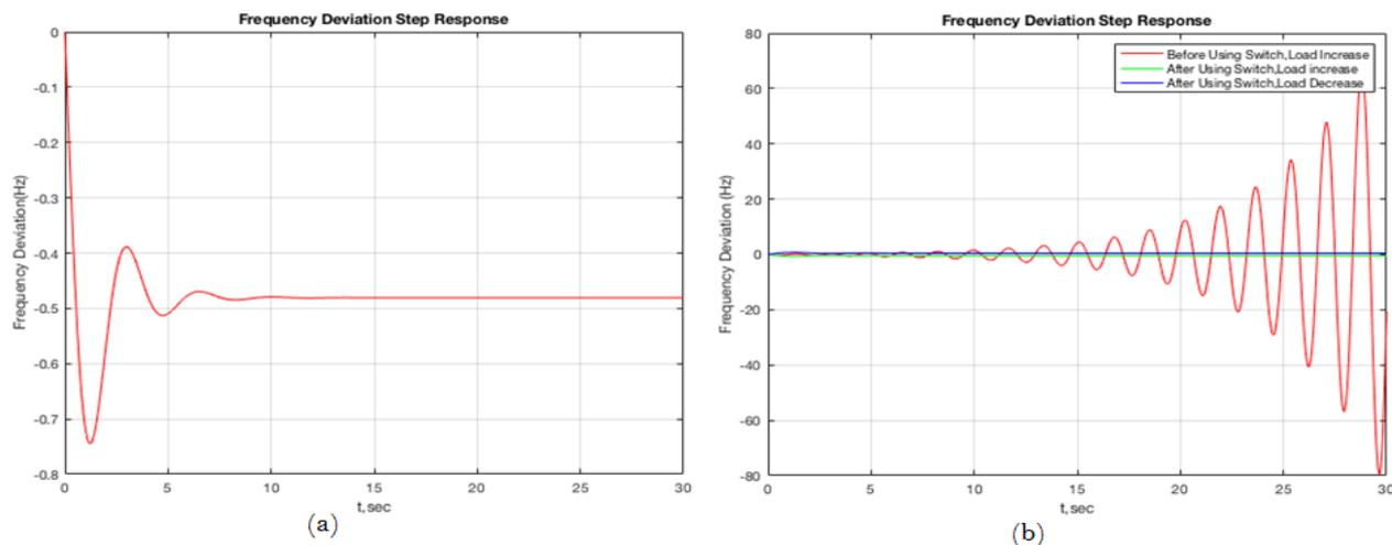
Figure-4. Frequency deviation step response for determining (a) frequency deviation step response under sudden load increase (b) frequency deviation step response using switch in LFC loop under sudden load change.
