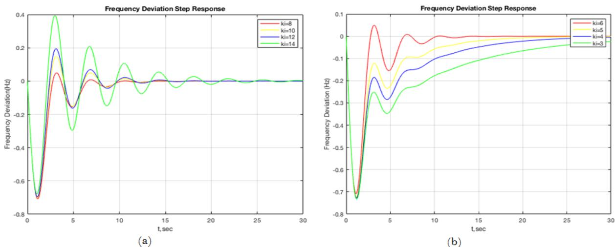
Figure-3. Frequency deviation step response for determining (a) frequency deviation for AGC under positively biased attack condition (b) frequency deviation for AGC under negatively biased attack condition.
