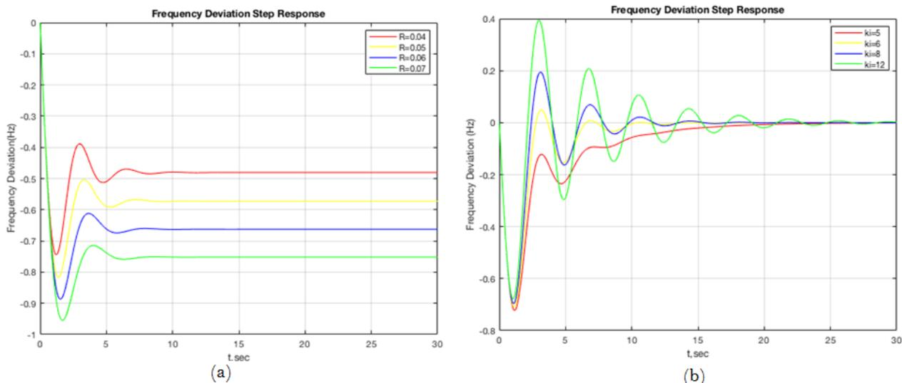
Figure-2. Frequency deviation step response for (a) LFC under negatively biased attack condition (b) determining frequency deviation step response for AGC.
