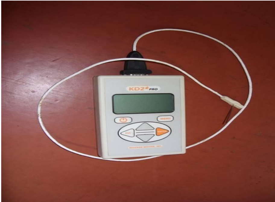
Figure-4. Single-needle sensors for thermal conductivity and resistivity measurements (6 cm) for liquids
