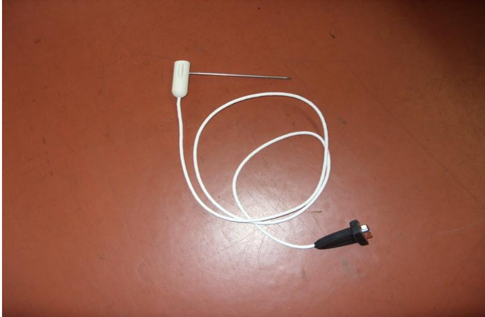
Figure-5. Extended single-needle sensors for thermal conductivity and resistivity measurements (10 cm) for use in hard materials
