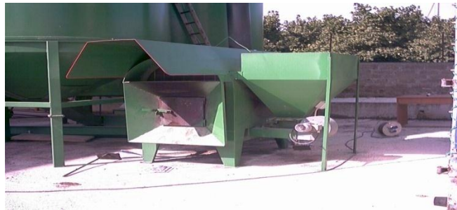
Figure-7. Production Nutshell and pruning (biomass)/solid fuel boiler applied to a dryer
