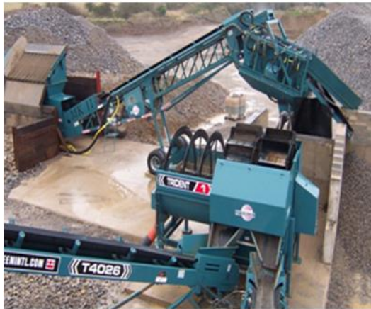
Fig-25. Washing Plant in operation (left) and Power screen (Right)
