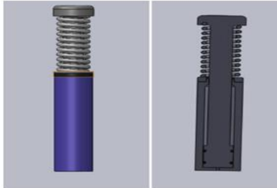
Figure-2. Internal Structure of the Air pump Source: Ibrahim (2014)
