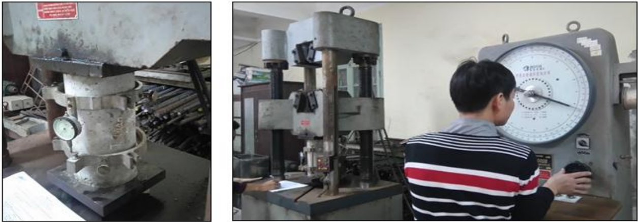
Figure-6. Modulus of elasticity test set up.
