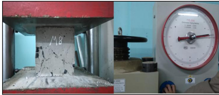
Figure-4. Compressive strength test set up.
