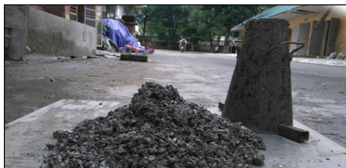
Figure-3. Slump test set up.
