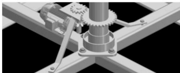
Figure-4. Sun tracking PV system and enlarged view of the drive mechanism.
