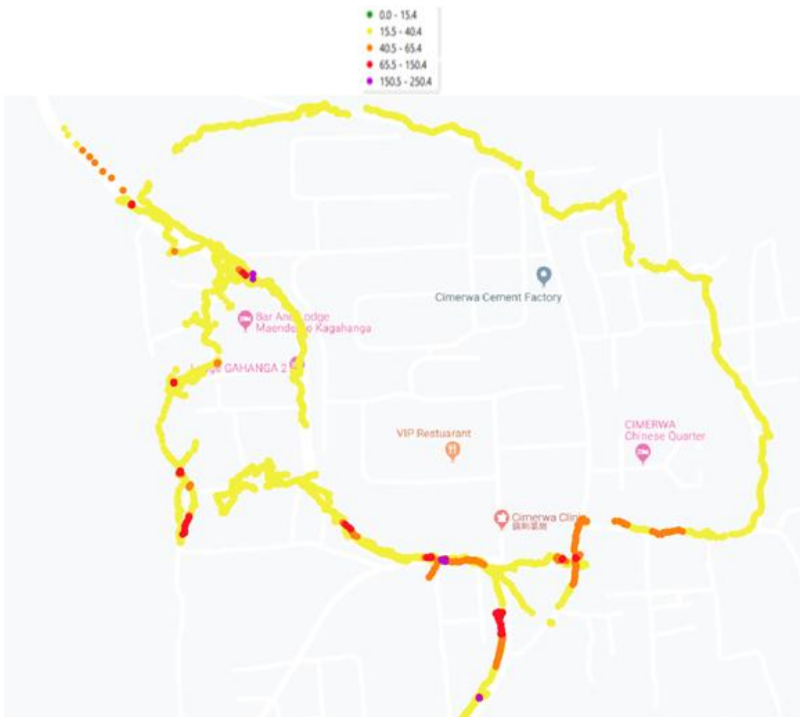
Figure-13. Distribution levels of PM 2.5 pollutant in factory surrounding areas for a random walk during sampling activities. The PM 2.5 concentration levels for such walk are represented by different colors Table-3. This Figure indicates that high level of PM 2.5 is located at CIMERWA Clinic and Lodge GAHANGA-2 and in the road from the factory to MASHESHA center.
