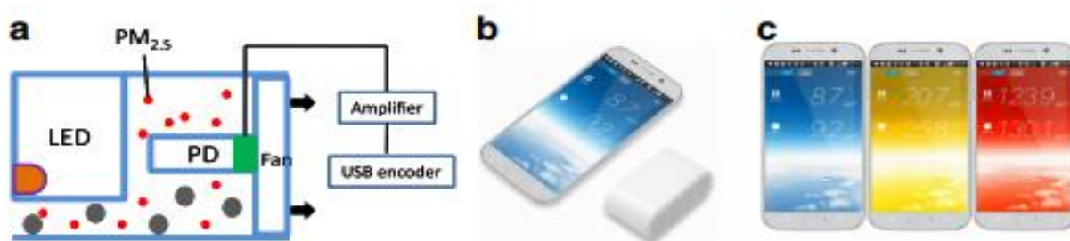
Figure-4. Pocket PM 2.5 Sensor. a) Principle of Pocket PM 2.5 Sensor Module, LED, light-emitting diode; PD photodiode; USB, Universal Serial Bus. b) Pocket PM 2.5 Sensor connected to a smart phone with android system. c) Color variations for different levels of PM 2.5 concentration. Source : Yi et al. (2018).
