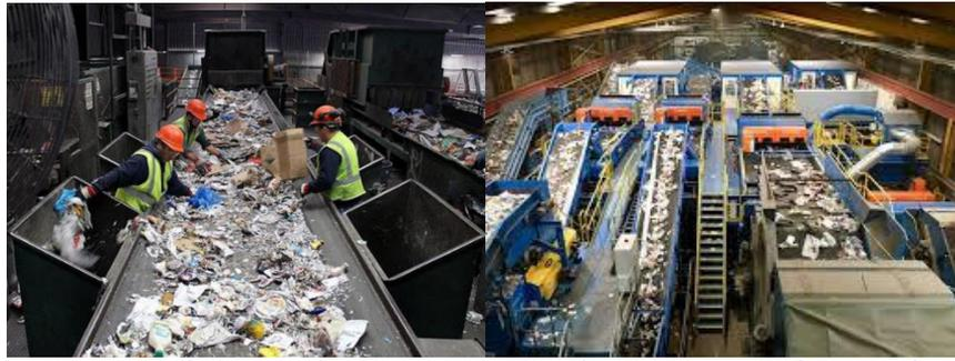
Figure-7. Further sorting of waste at processing/transfer station (Manual and Automated).
