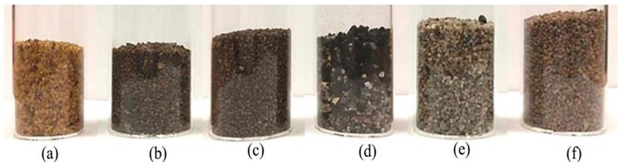
**Figure 1.** Bed samples from each biomass; (a) fresh sand (b) palm fronds (c) domestic wood (d) corn straw (e) sugarcane bagasse (f) plantain peels.
