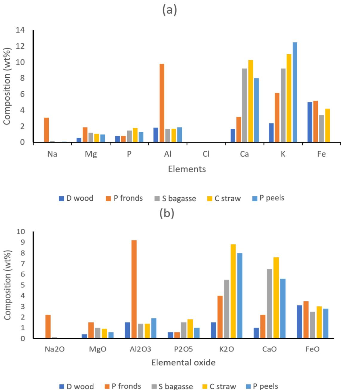
Figure 2. XRF analysis of bed samples obtained from different biomass fuels under air combustion; (a) elemental composition and (b) elemental oxides. Results are given as C and O free basis.
