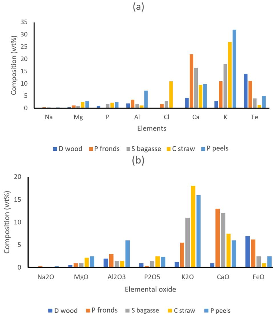
Figure 4. The XRF results for biomass ash under air combustion; (a) elemental composition and (b) elemental oxides. (Presented results are Si free basis).
