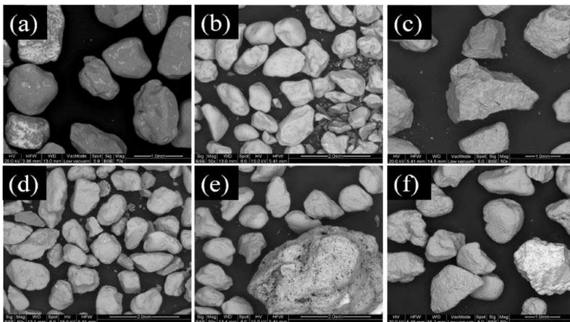
**Figure 5.** SEM micrographs of bed sample; (a) fresh sand, (b) domestic wood, (c) palm fronds, (d) sugarcane bagasse, (e) corn straw and (f) plantain peels.
