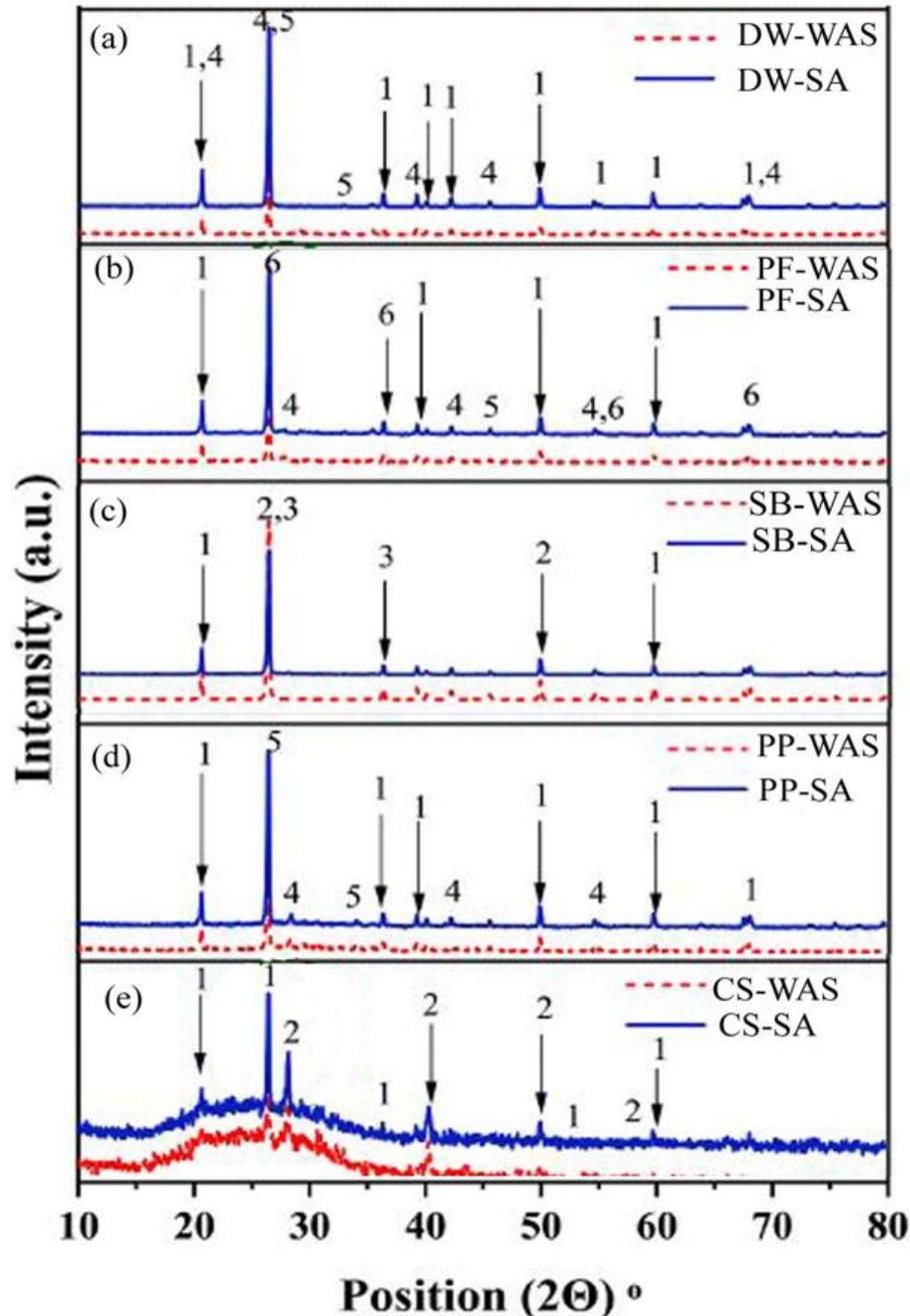
**Figure 3.** XRD spectrum of different biomass (DW-domestic wood; PF-palm fronds shell; SB-sugarcane bagasse; PP- plantain peels; CS-corn straw) under; (a) staging air (SA) and without air staging (WAS) conditions. (1. Quartz, 2. Sylvite, 3. Sodium phosphate hydrogen peroxide, 4. Coesite, 5. Hematite and 6. Albite).
