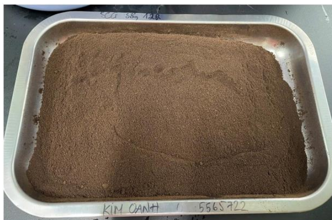
Figure 1. Dried SCG sample after oven-drying at 105 °C for 12 hours.
