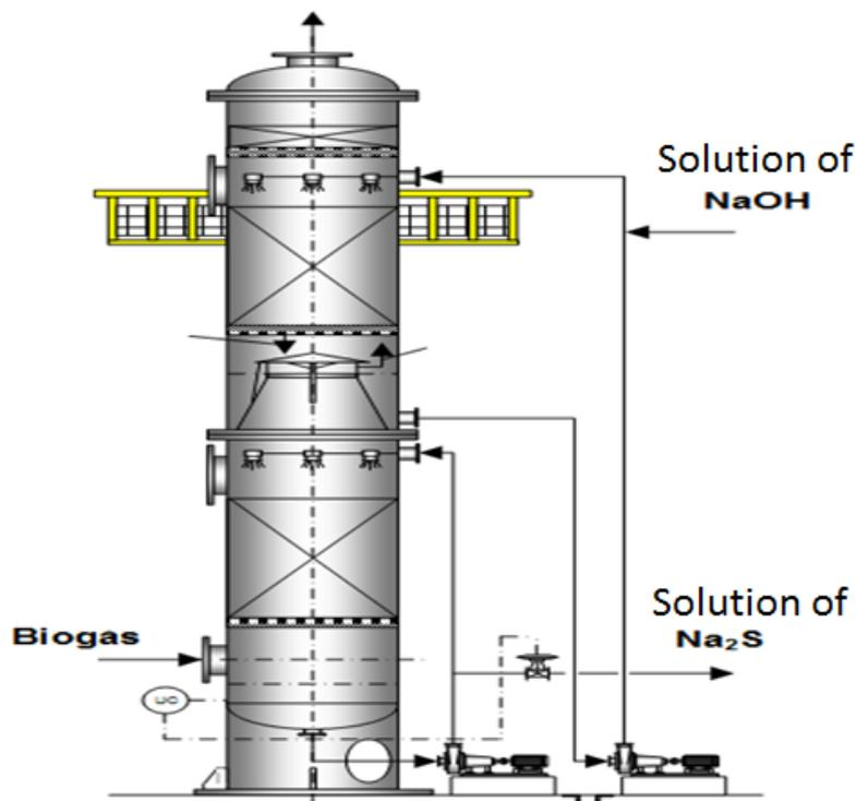
Figure-2. Packing tower details.
