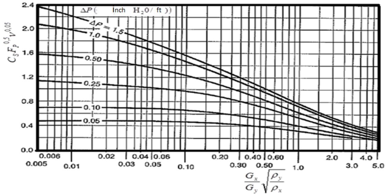
Figure-1. Correlation to widespread flooding and loss of pressure in columns.
