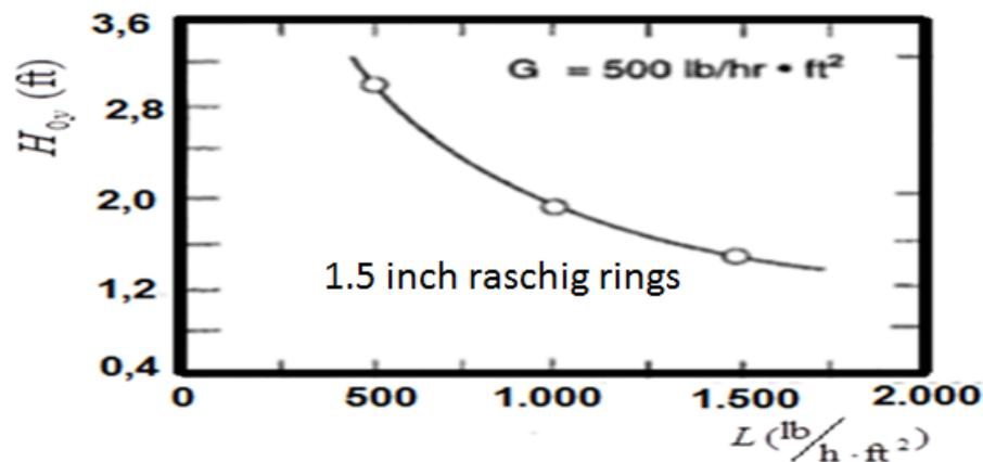
Figure-3. Transfer unit height (Norman, 1962).
