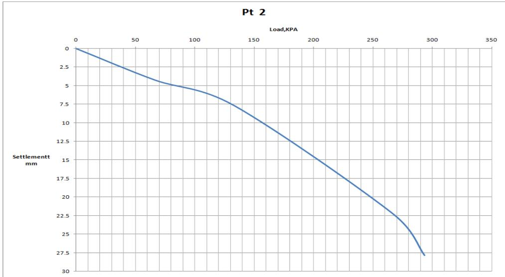
Fig-8. Loading settlement plot for point 2
