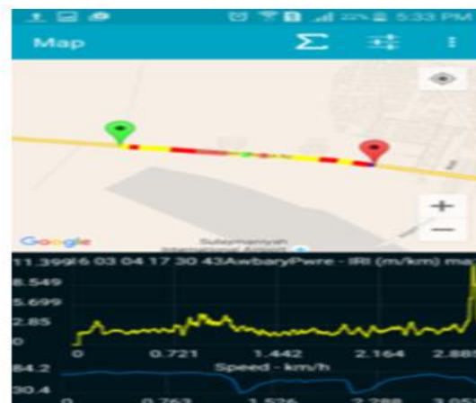
Fig-8. Map with IRI graph. (collected by authors) Screenshot of the application used for collecting data using IRI moving average graph which uses a variable sized average.
