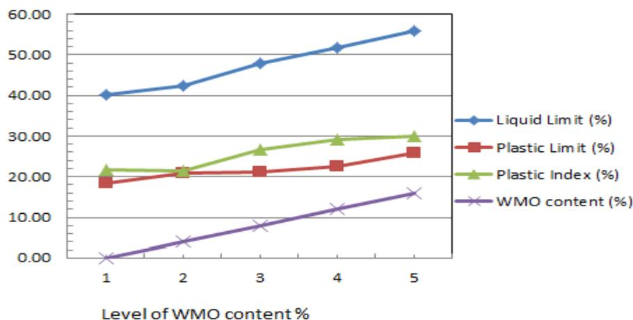
Figure-4. 1. Atterberg Limit for Clay Soil
