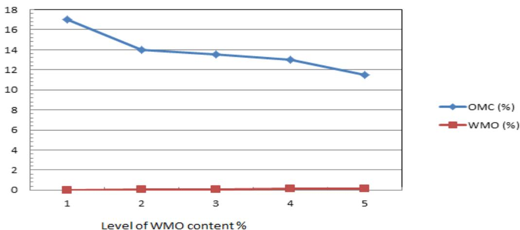
**Figure-4.4.** Optimum Moisture Content (OMC) for Clay Soil
