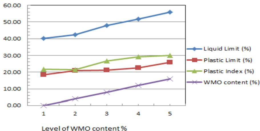
Figure-4. 1. Atterberg Limit for Clay Soil
