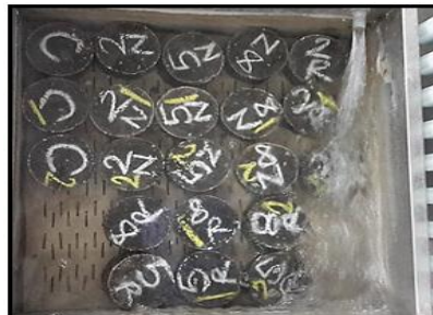
Samples placed in distilled water Fig-9. Indirect Tensile Test
