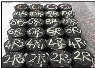
Samples prepared by Marshall Mix Design
