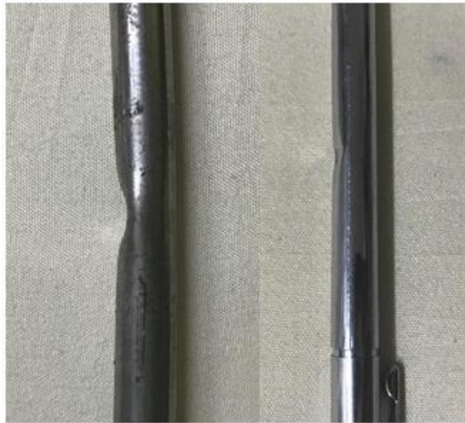
Figure-10. Deformation of the cylindrical object impacted by the bullet at the edge of the circumference (left) and the stainless steel pen impacted by the bullet at the edge of the circumference (right).
