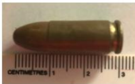
Figure-7. 9 mm FMJ bullet with copper gilding.
