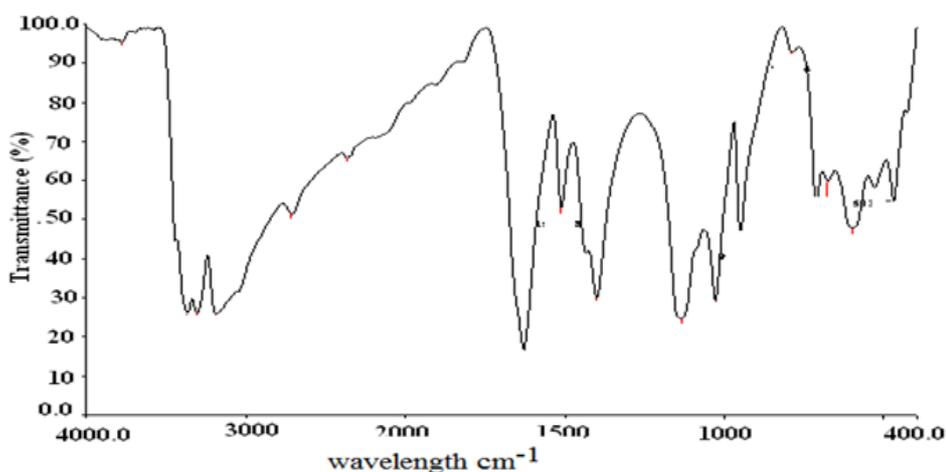
Fig-2. FTIR spectrum of BTSZS crystal
