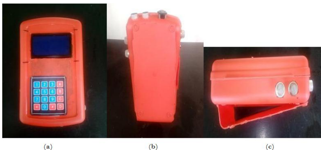
Figure-2. Petroleum Product Volume Estimator and Tracker (PPVET) [15] (a) Front View (b) Back View (c) Side View.
