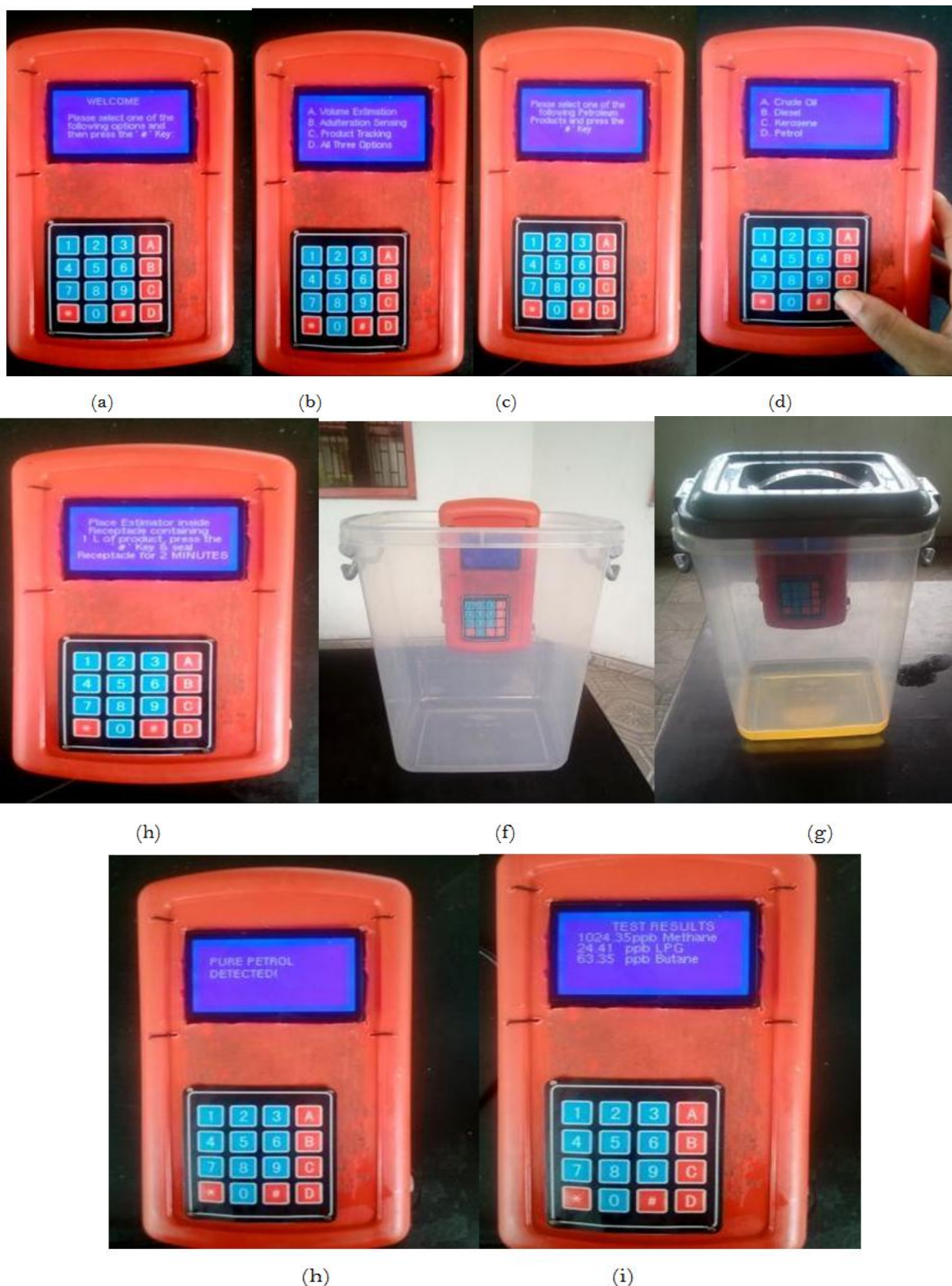
Figure-4. GVE test on unadulterated petrol sample from NNPC Retail Outlet. (a) PPVET welcome message asking user to select a function to perform (b) PPVET listing available functions, including Adulteration Sensing (c) User is asked to select a type of petroleum product for Adulteration detection (d) Options available for Adulteration Sensing (e) Instructions to commence Adulteration Sensing (f) Setup for GVE test (g) GVE test in progress (h) Result of GVE test on pure petrol sample (i) GVE gas concentration measured during the test.
