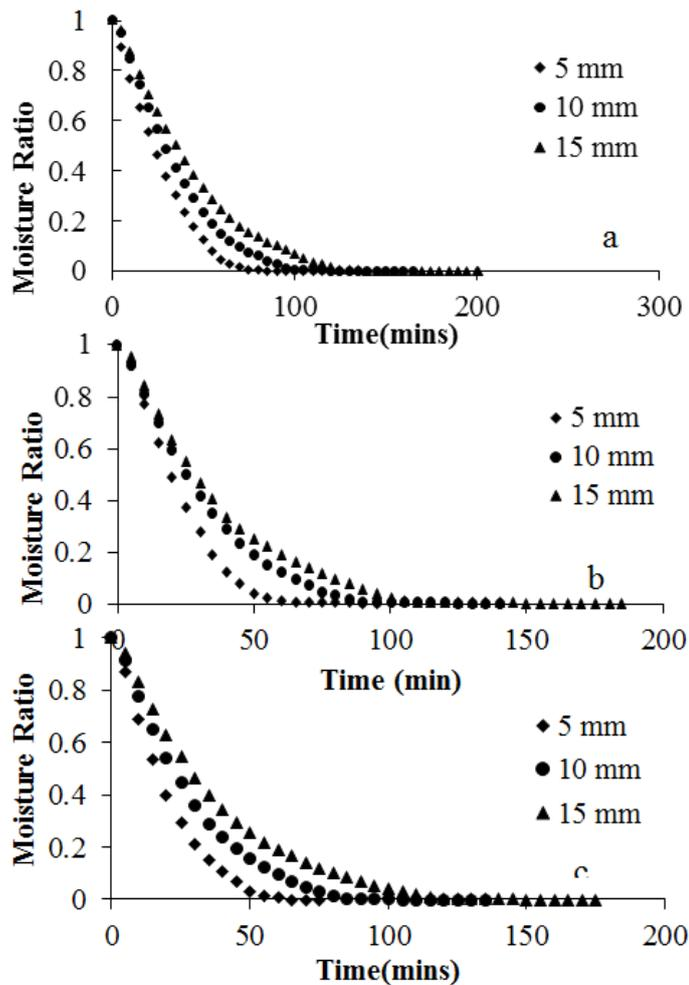
Figure-2. Moisture Ratio vs. Time at temperature (a) 90°C, (b) 100°C and (c) 110°C.
