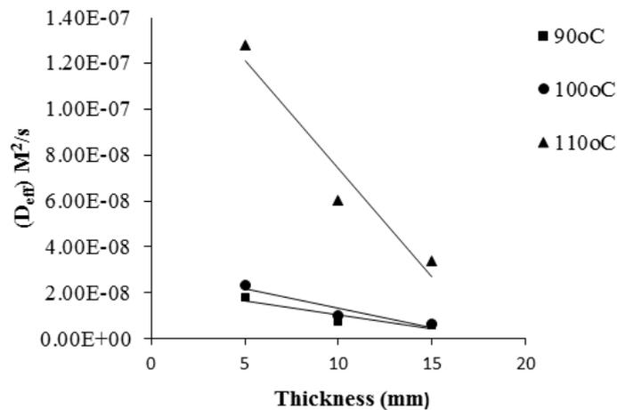
Figure-4. Effective moisture diffusivity versus thickness.
