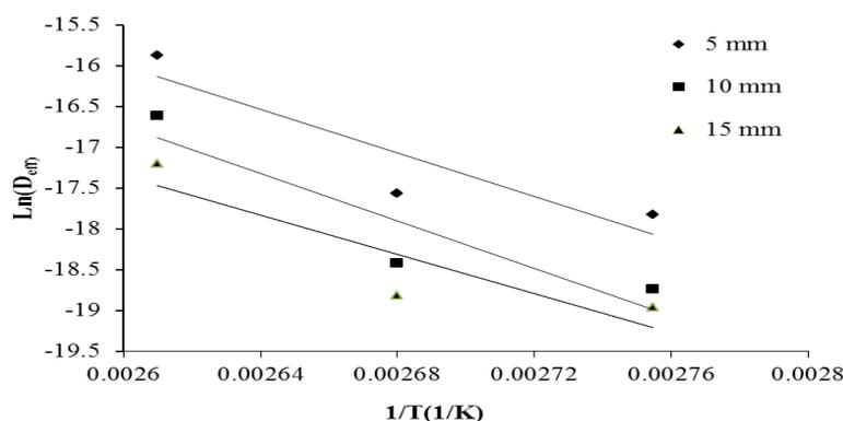
Figure-5. The effect of temperature and effective moisture diffusivity of okra.
