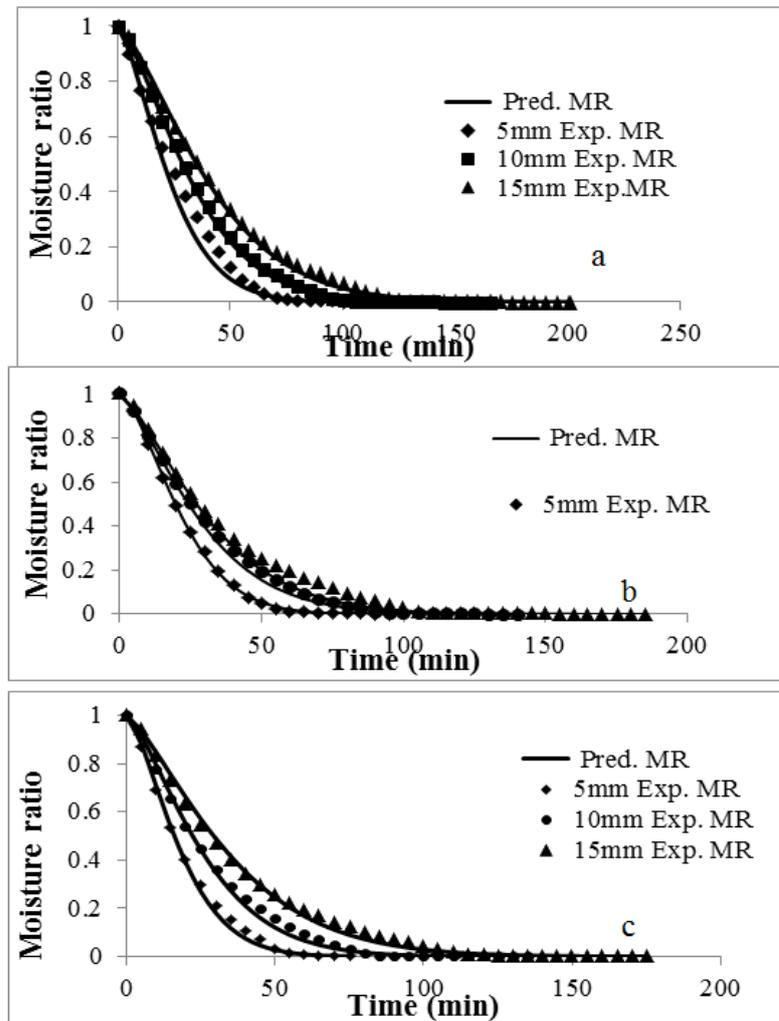
Figure-3. Page's Model for thin layer drying of okra at (a) 90°C, (b) 100°C and (c) 110°C for 5mm, 10mm and 15mm thickness.
