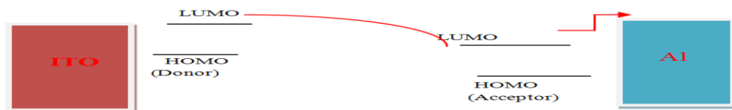
Figure-5. The donor-acceptor components in bulk heterojunction photovoltaic cell architecture (Kiesboms et al. , 2001; Peng et al. , 2008; Thompson and Frchet, 2008).
