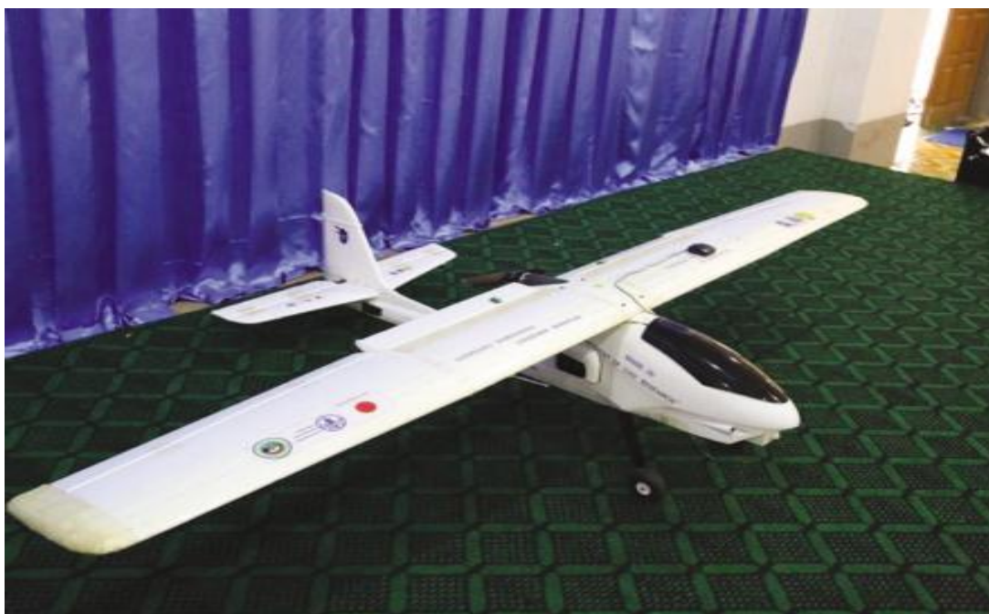
Figure-5. Wing drone which used for mapping rural areas in the Republic of the Union of Myanmar [1]. Source: Food and Agriculture Organization of the United Nations (FAO) [1].
