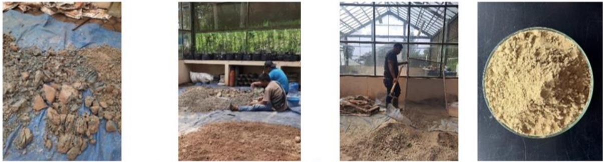
A) Dewatering of the tailing B) Grinding process of the tailing C) Tailing sieving D) Sieved tailing
