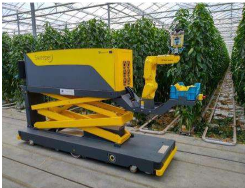
Figure 12. SWEEPER robotic system for sweet pepper harvesting.
