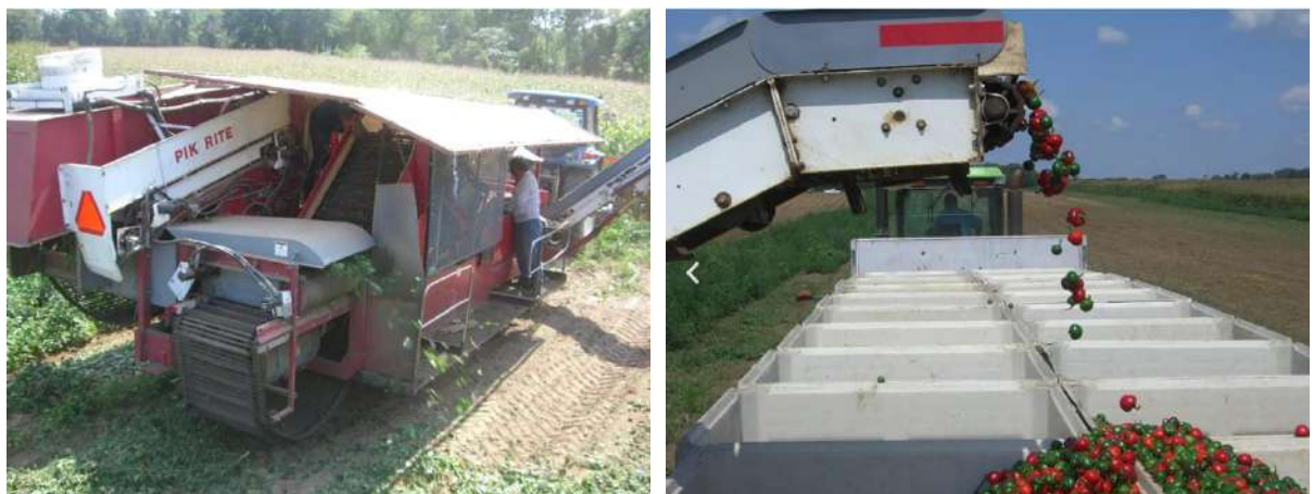
Figure 9. Capsicum harvesting using the Pik Rite pepper harvester.
