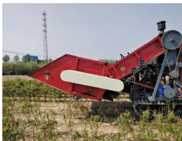
b) Pod-pepper-picking drum mechanism.
