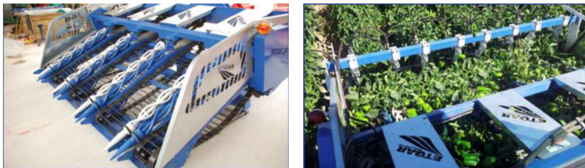
Figure 10. Operation of the Elad Etgar Series 2000 bell pepper harvester.
