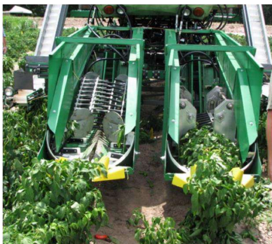
a) Spring-finger roller-type mechanism.
