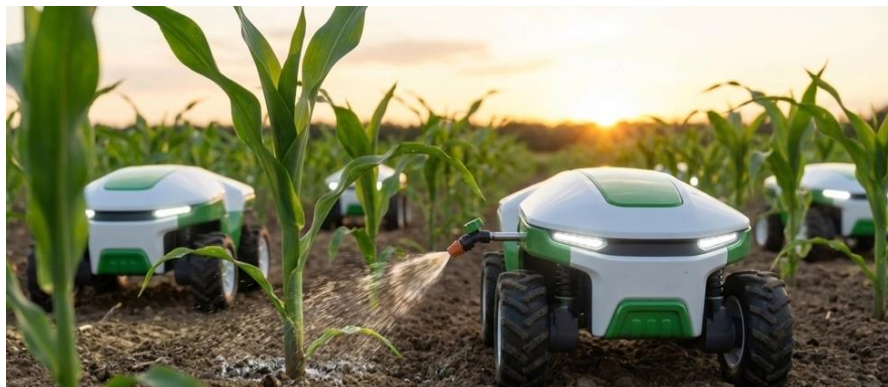
Figure 2. Smaller, lightweight autonomous electric platforms address soil compaction and labor shortages with 24/7 operation.
