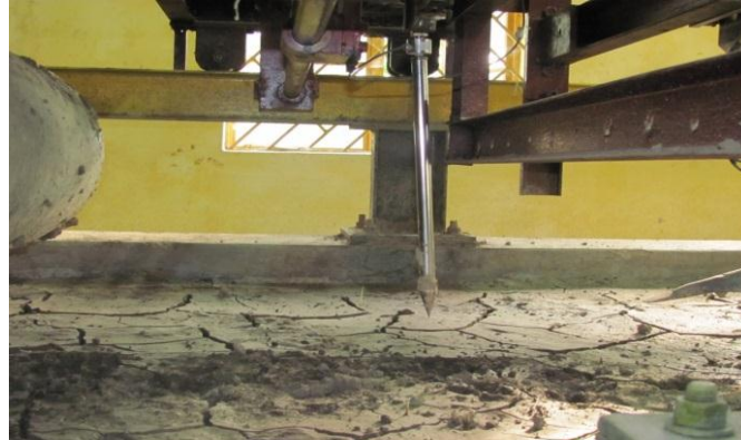
Fig-3. Cone penetrometer attached with soil processing trolley
