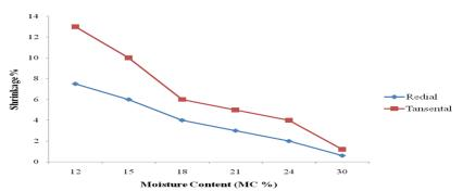
Figure-2. Graphical Relationship between Shrinkage and Moisture Content of K. senegalensis wood.
