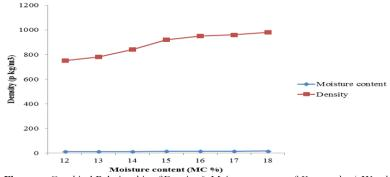
Figure-1. Graphical Relationship of Density & Moisture content of K. senegalensis Wood.
