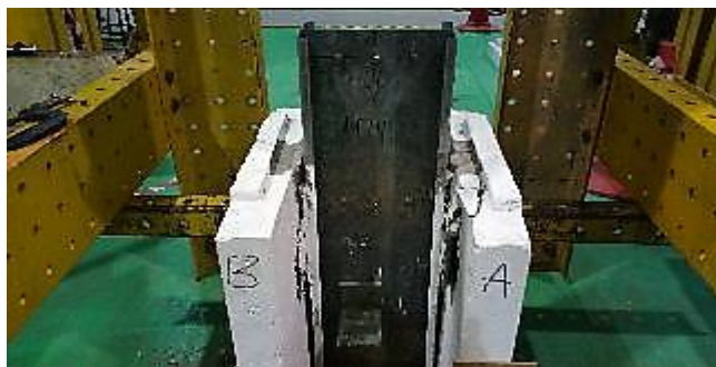
Figure-7. Failure mode of S4M14 test specimen
