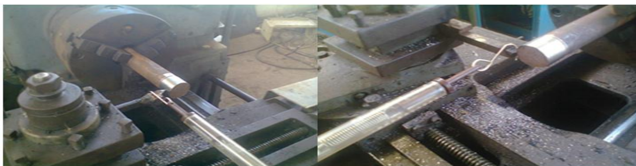
Figure-4. Dry turning test and feed cutting force measurement using dynamometer
